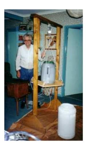
The platform is lowered to the floor, and a 25lt or 30lt container of wine is dragged onto the platform, and then by pulling the rope, the platform is raised high enough to allow me to slide under it a light but strong table that is placed ready, see at the left of the photograph.
