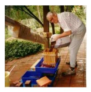
The basket is stood in a plastic tray with a hole in one corner, raised on a wooden platform high enough to allow a smaller plastic tray to catch the juice. After filling the basket with grapes, the square board is placed on top, and then the required number of blocks to fill the space up to the press lever arm.
